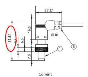
Reason for change: To enhance the reliability of the wiring process prior to injection molding.
